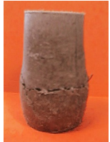
Unsaturated Triaxial Tests, Confined at 5 psi (34.5 kPa)
